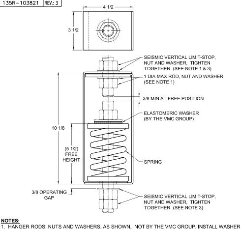
.134 THK, MIN, X 2 O.D. MIN WITH REQUIRED INSIDE DIAMETER TO ACCOMMODATE ROD SIZE IN USE.
